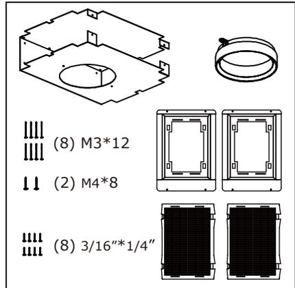
ZRC-02RM includes (1) additional filter and bracket with screws.
