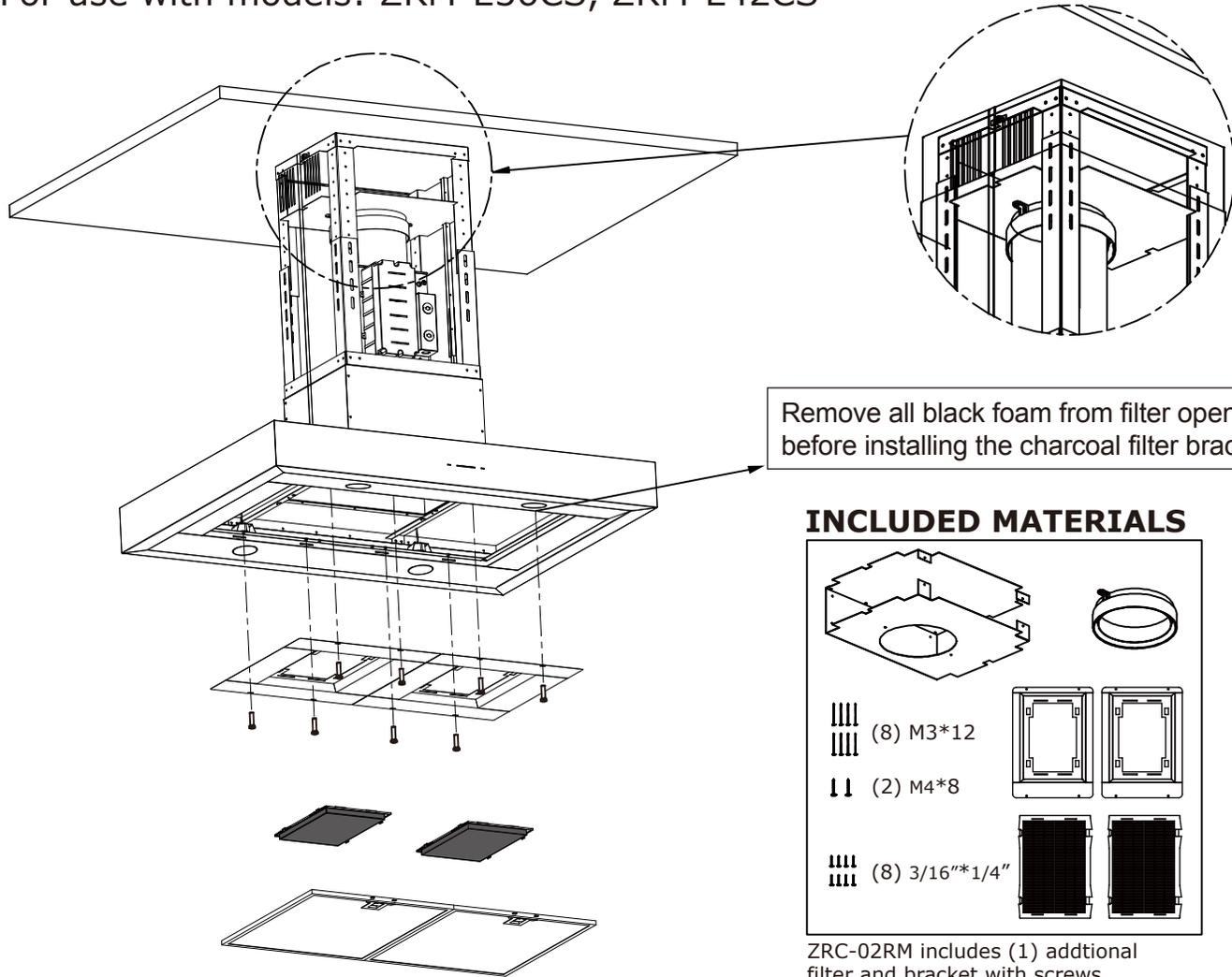
Remove all black foam from filter opening before installing the charcoal filter brackets.
