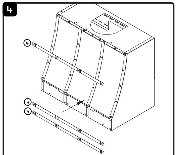
See Forte hood installation instructions for more installation details. Use the bushings, washers, and wingnuts inside the Hood Banding Hardware packet, included with the hood, to complete assembly.
