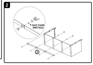
See Forte hood installation instructions for more installation details. Use the washers and wingnuts inside the Duct Cover Hardware packet, included with the duct cover, to complete assembly.
