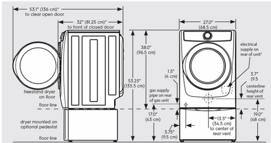
\* Connection of water inlet hose on steam dryer adds 3/4 in. (2 cm) to installation depth.
