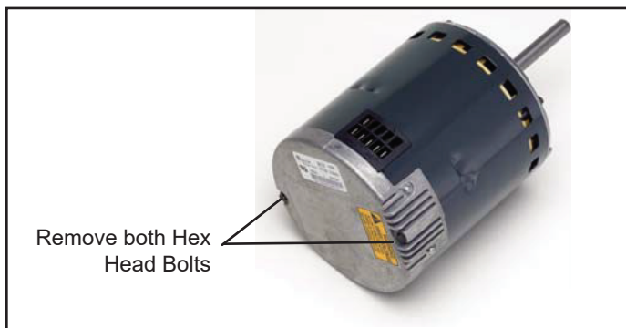
Figure 13. Remove the Hex Head Bolts
