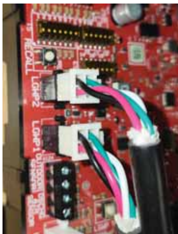
Figure 45. Modulating Furnace Control
