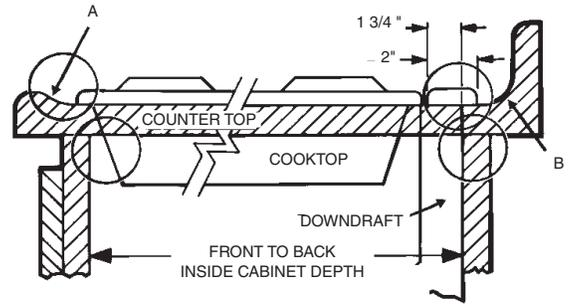
Refer to the cooktop installation instructions for dimensions of cooktop, countertop cut-out, and cabinet requirements. The RMDD3004EX can be installed in most standard 30" wide cabinets, (RMDD3604EX can be installed in most standard 36" wide cabinets), (RMDD4804EX can be installed in most standard 48" wide cabinets).
