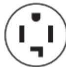
4-wire receptacle (14-30R)
