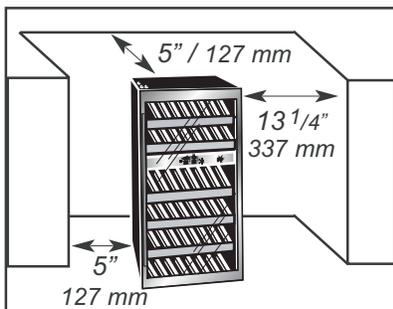
**Allow 13 1/4" (33.7 cm) of space** between the (hinge) side of the door and any adjacent wall to accommodate door swing.
