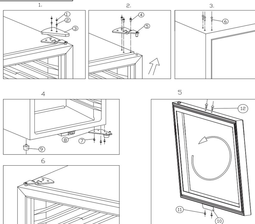
1. Close the door and take out rubber cover (1), unscrew two screws (2) and remove decorative cover (3). (Fig.1)
