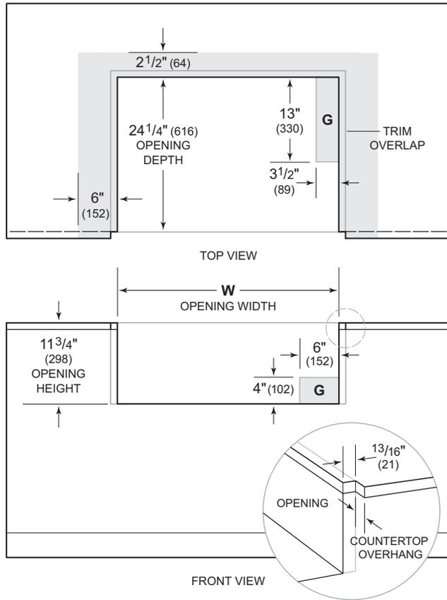
NOTE: Shaded area above countertop indicates minimum clearance to combustible surfaces, combustible materials cannot be located within this area.
