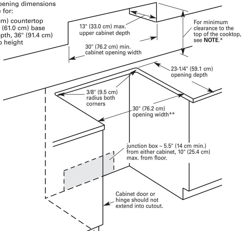
**\*NOTE:** 24" (61 cm) min. when bottom of wood or metal cabinet is protected by not less than 1/4" (6.4 mm) flame retardant millboard covered with not less than No. 28 MSG sheet steel, 0.015" (0.4 mm) stainless steel, 0.024" (0.6 mm) aluminum or 0.020" (0.5 mm) copper. 30" (76.2 cm) min. clearance between the top of the cooking platform and the bottom of an unprotected wood or metal cabinet.
