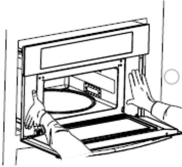
3. Using an 1/8" (3.2 mm) drill bit, predrill pilot holes through the mounting rails on each side of the microwave oven.
