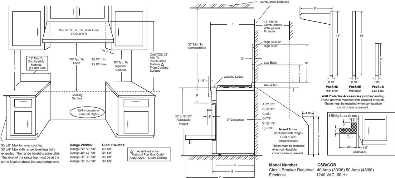
**GAS REQUIREMENTS:** 1/2" NPT gas connection. Minimum gas supply is 7" water column for natural gas and 11" for propane. Operating pressure at the manifold is 5" water column for natural gas and 10" for propane. All units include a gas regulator. The installer must provide a shut-off valve at the rear of the appliance with easy access to shut off the gas for service. High-altitude kits and gas conversion kits are available through the Capital parts department.
