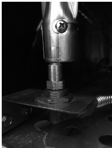
REAR BURNER NOT PROPERLY SEATED
