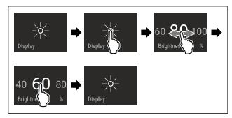
Fig. 36 Example illustration: Switching from 80 % to 60 %.
