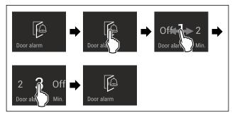
Fig. 38 Example illustration: Changing the door alarm from 1 minute to 3 minutes.
