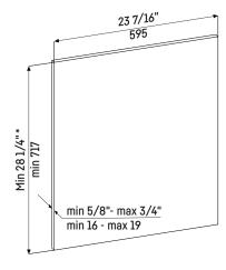
Custom panels should be at least 5/8"(16mm) and a maximum of 3/4"(19mm) thick.
