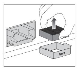
■ To **replace** a charcoal filter, remove the used charcoal filter from the retainer and dispose of the charcoal filter with normal household waste.
