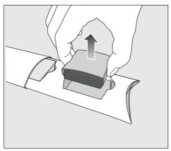
Take the charcoal filter out of its packaging together with the filter protection. Risk of damage as a result of incorrect handling.
