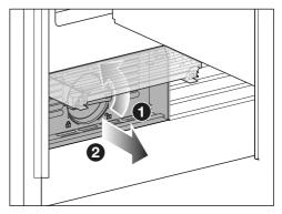
■ Turn the filter cartridge 90° counterclockwise until it is in the vertical position 1 and slide it out 2.
