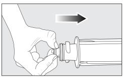
Reinsert the mesh filter into the filter cartridge.
