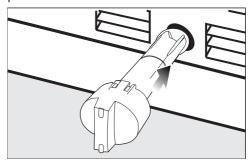
■ Slide the new filter cartridge or the mesh filter into the filter opening as far as it will go, making sure the cap is vertical.
