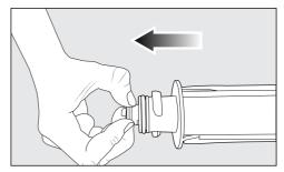
■ Pull the mesh filter out of the filter cartridge.
