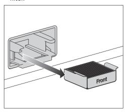
Pull the used charcoal filters and their retainer out of the holder.
