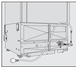
■ Insert the plug into the back of the appliance.
