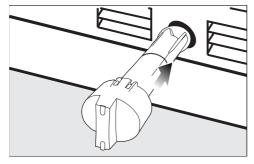
Slide the filter cartridge into the filter opening, making sure the cap is vertical.
