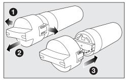
■ Loosen the cap from the old filter cartridge **①** and pull the cap off **②**.
