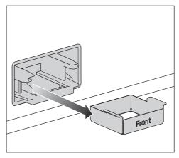
Remove the retainer for the charcoal filter from the holder.
