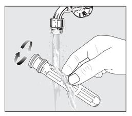
Rinse the mesh filter under running lukewarm water. Turn the mesh filter over under the running water to clean it on all sides.
