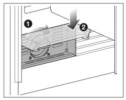
■ Turn the filter cartridge clockwise 90° as far as it will go until it is in the horizontal position ①.
